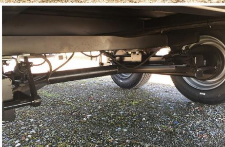
Dim. : 7m00 x 2m54, Ressort Flèche + protection, Balancier Monroc, RC 245/70 R19.5 + RS, Rampes Larges...
