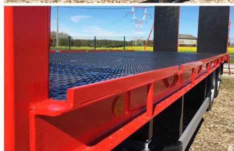
Dim. : 7m00 x 2m54, Ressort Flèche + protection, Balancier Monroc, RC 245/70 R19.5 + RS, Rampes Larges...
